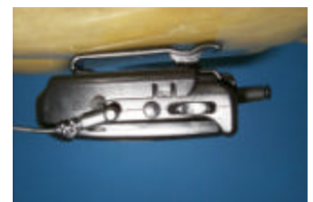
Figure 13. Body Holster Configuration
