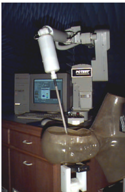
Figure 5. Photograph of the Probe and the Phantom
