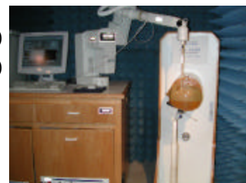
Fig. 1 SAR Test Setup
