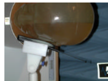
Figure 14. Head SAR Test Setup
