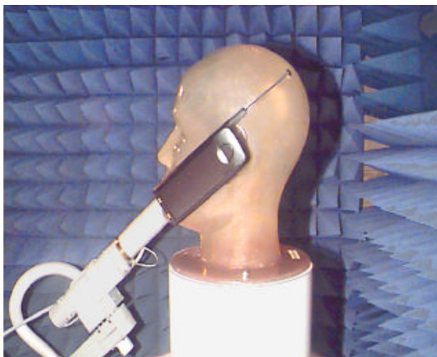
Figure 9. Sample of Handset alignment with the Ear Canal of the Phantom
