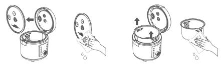
3.Use a clean cloth to clean the exterior pot of the rice cooker. Pay special attention to clean the groove surrounding the heating element.
