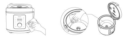
4.Detach and wash the condensation collector.
