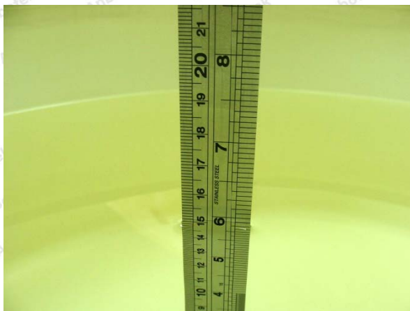
Photo of Liquid Height for Body SAR
