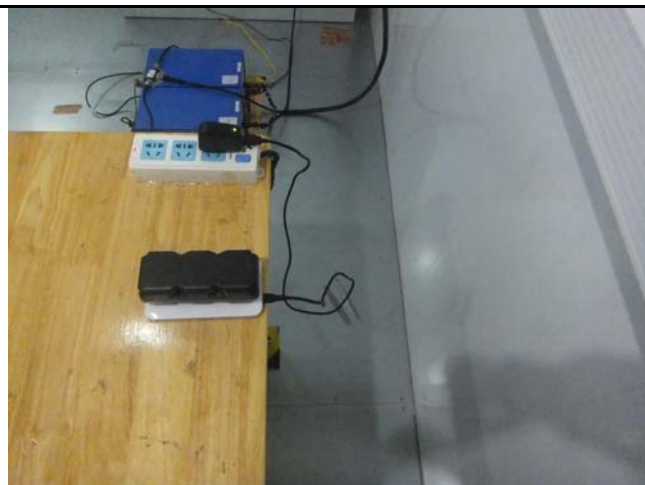
Conducted Emissions Test Setup – Side View
