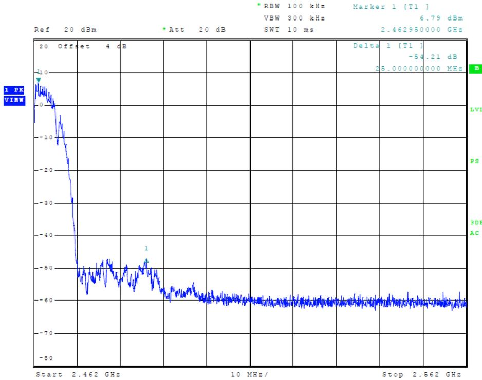
**Figure 9 Plot of Transmitter High Band Edge (802.11b)**
