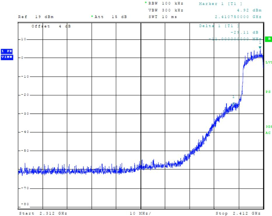
**Figure 7 Plot of Transmitter Low Band Edge (802.11g)**
