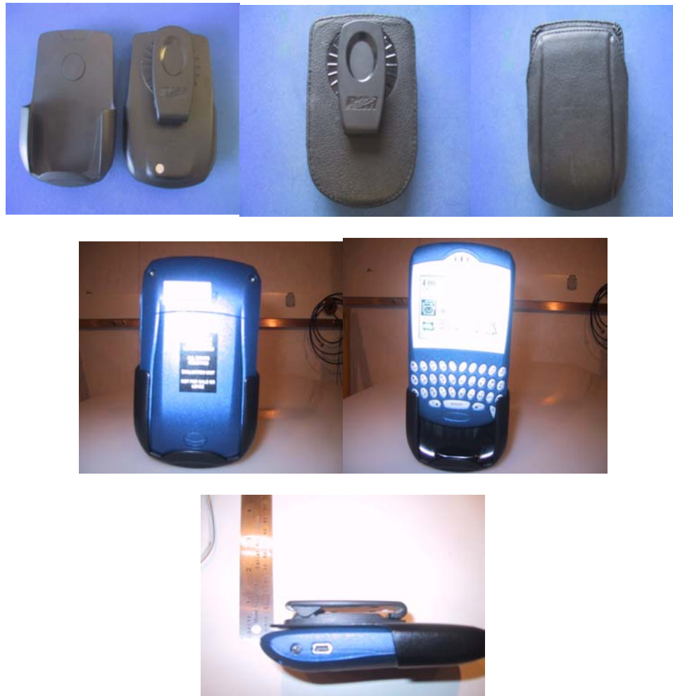
Figure 2. Body-worn Holster ASY-03998-001 and Leather Swivel Holster HDW-05400-001
