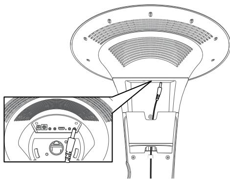
2 Connect the external device by using an appropriate cable (3.5mm audio cable not included) to the **LINE IN Jack** on the rear of this unit as previous described. Connecting an external unit will allow the audio to be played through your Singing Machine.
