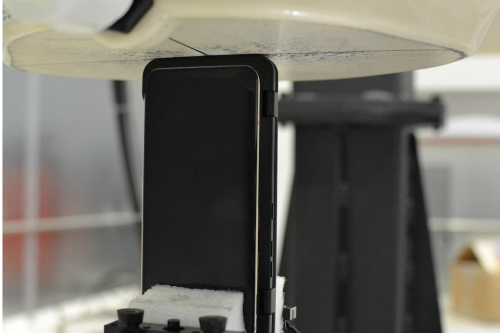
SAR Test Setup Photo 23 – Bottom Edge at 0 mm with Dual Display Cover Position 3
