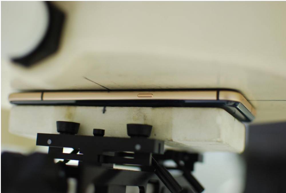
SAR Test Setup Photo 14 – Front Side at 1 mm
