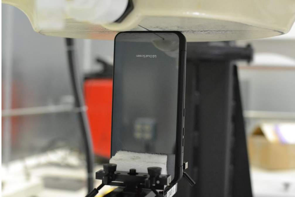
SAR Test Setup Photo 21 – Bottom Edge at 0 mm with Dual Display Cover Position 1
