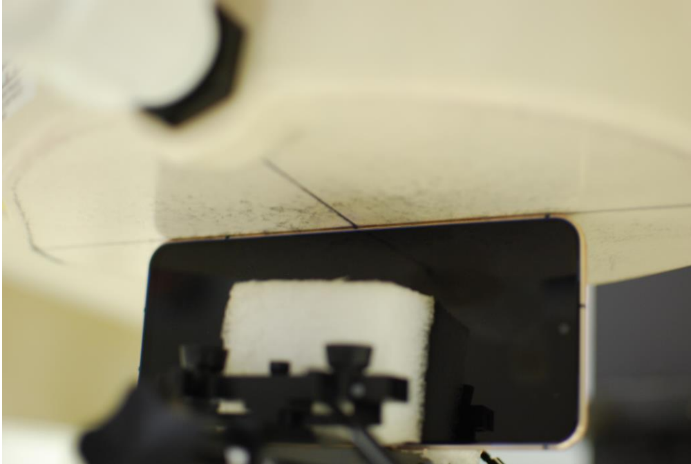
SAR Test Setup Photo 27 – Left Edge at 0 mm
