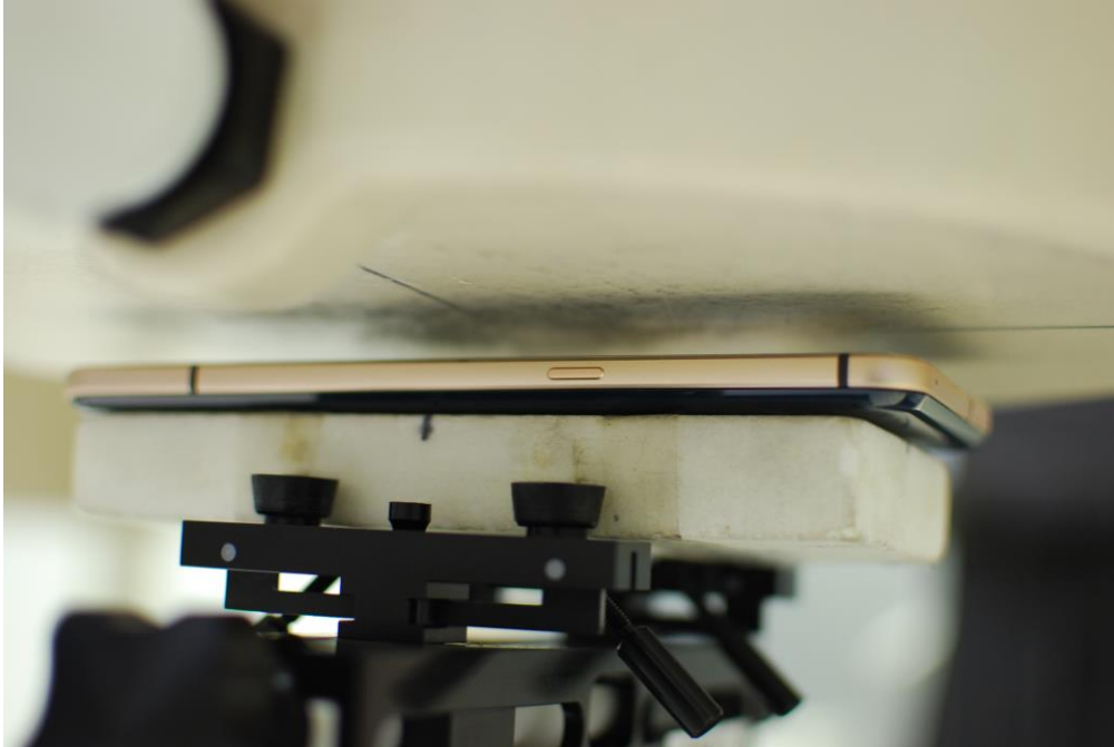
SAR Test Setup Photo 13 – Front Side at 10 mm
