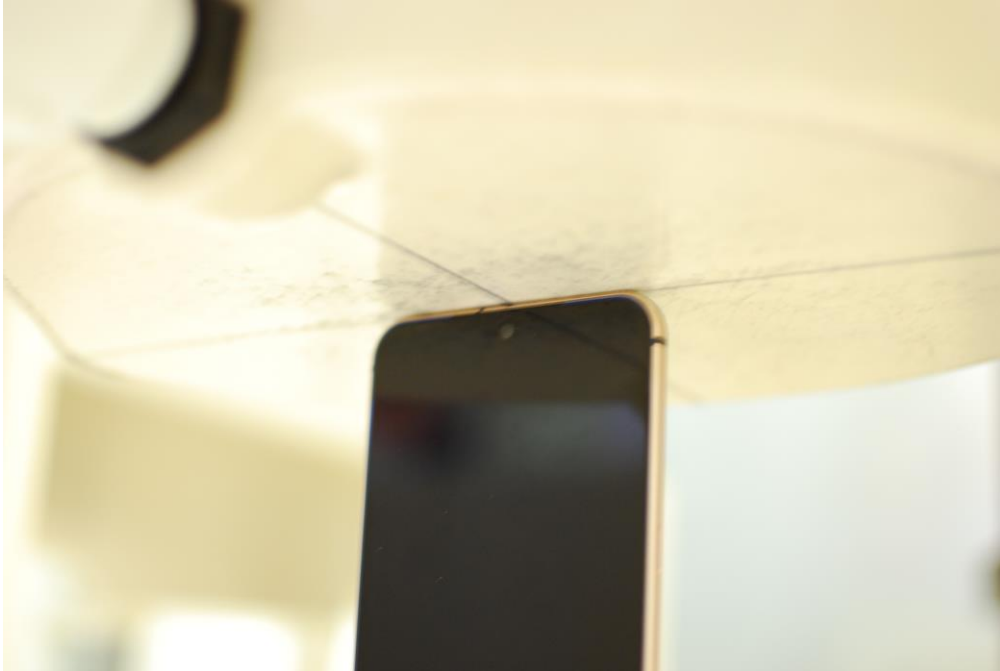
SAR Test Setup Photo 17 – Top Edge at 0 mm
