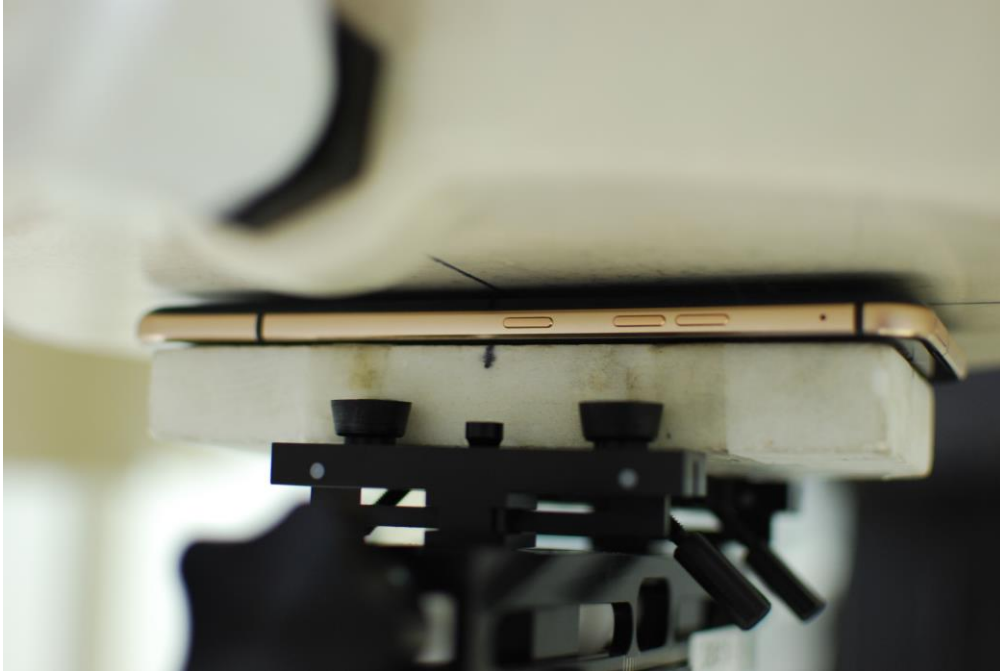
SAR Test Setup Photo 11 – Back Side at 2 mm
