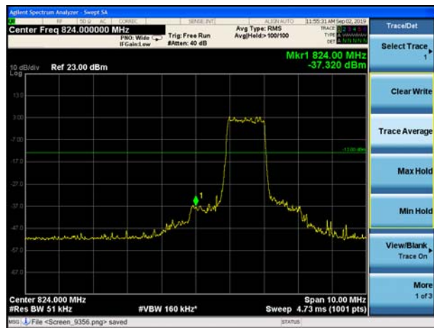
LTE Band 26 16QAM 1.4MHz CH-Low 1RB
