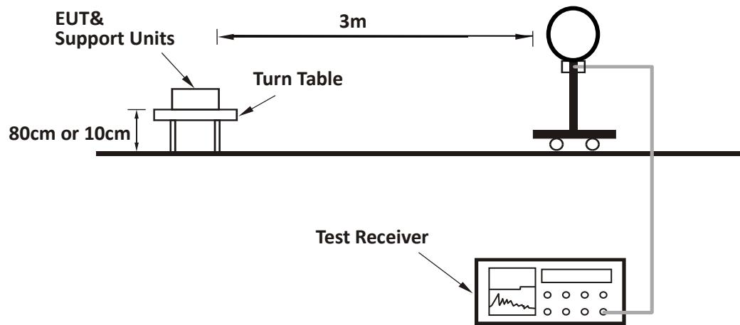
**For Radiated emission 30MHz to 1GHz:**
