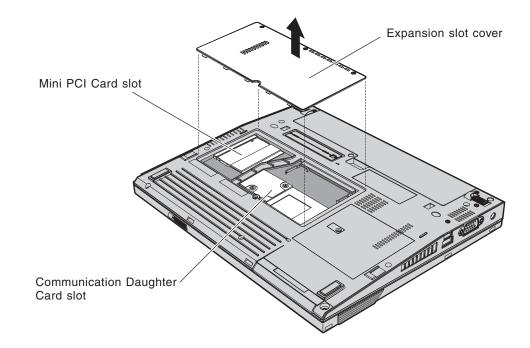
**Attention:** The ThinkPad X40 Series computer contains an authentication mechanism You can install or remove each wireless feature by yourself. If you install an unauthorized wireless adapter that is not approved for use in the ThinkPad X40 Series computer, the computer will not start, but only displays an error message and emits beeps.
