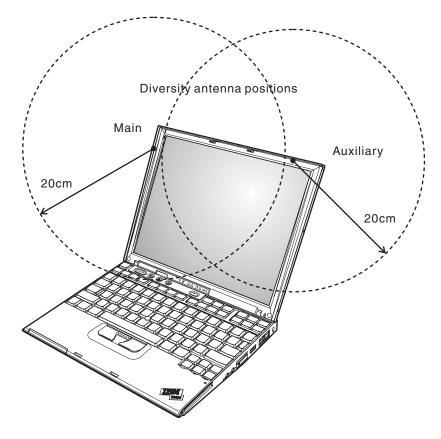
**Note:** The transmission diversity function is implemented for the cards listed above (models WM3B2200BG, WM3B2915ABG, T60H786-U, AR5BMB-44). The function does not emit radio frequencies simultaneously from both antennas. One of the antennas is selected automatically or manually (by users) to have good quality of radiocommunication.
