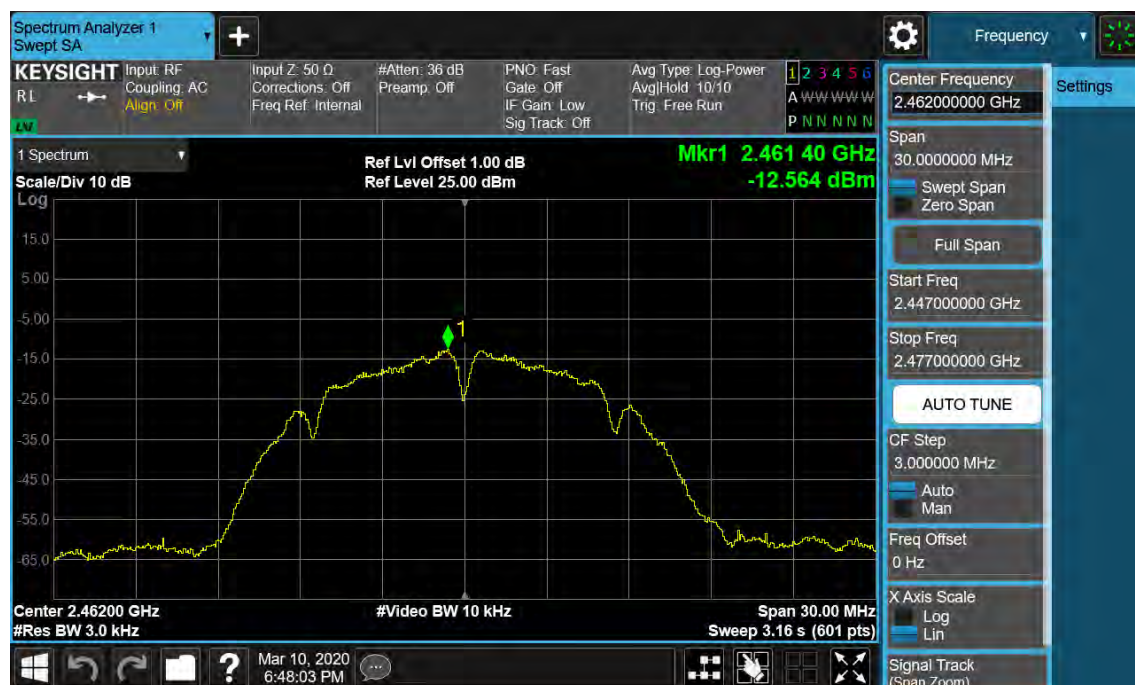
Figure 12: Power Spectral Density, 802.11b, 2462MHz
