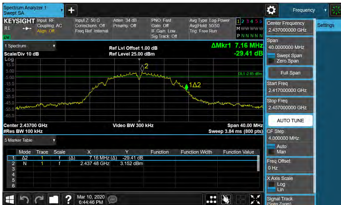
Figure 2: 6dB Bandwidth and 99% Bandwidth, 802.11b, 2437MHz
