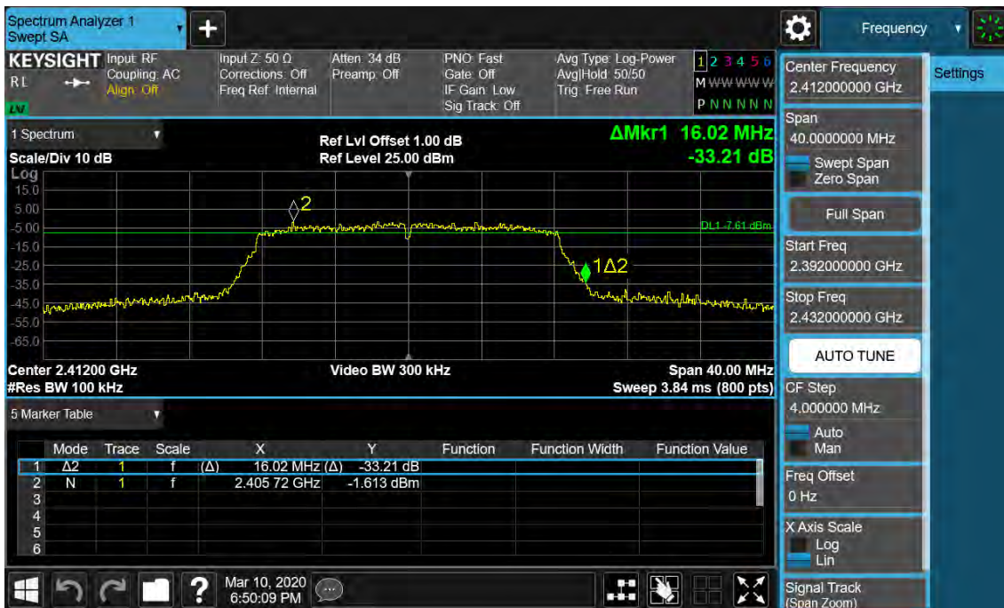
Figure 4: 6dB Bandwidth and 99% Bandwidth, 802.11g, 2412MHz
