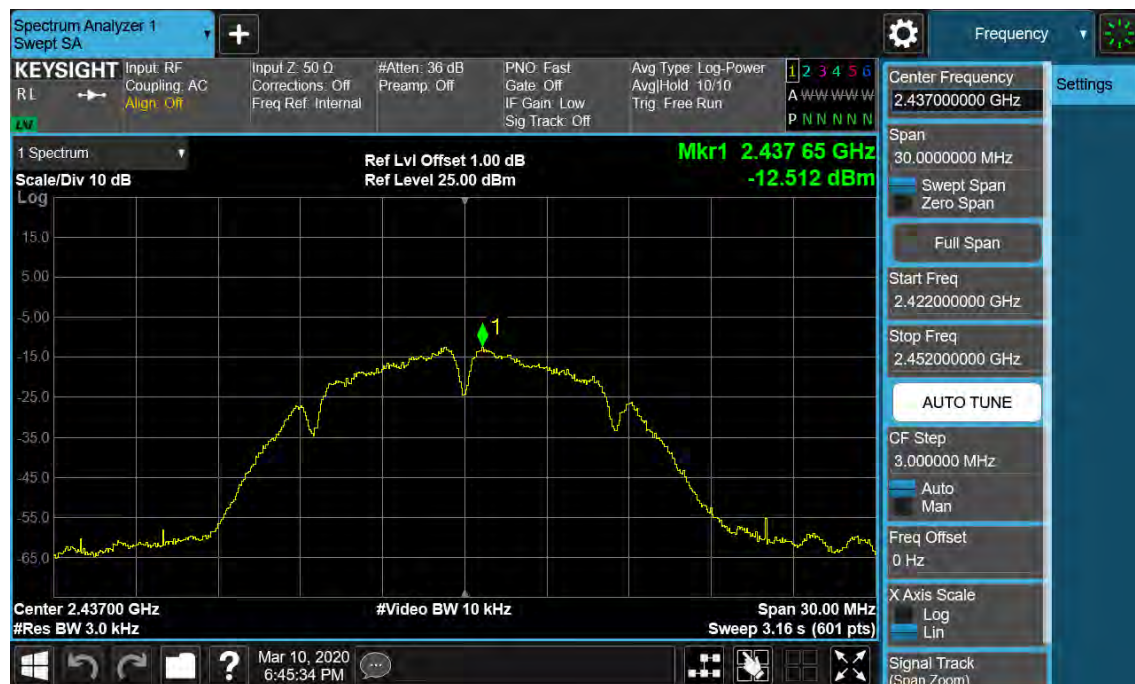
Figure 11: Power Spectral Density, 802.11b, 2437MHz
