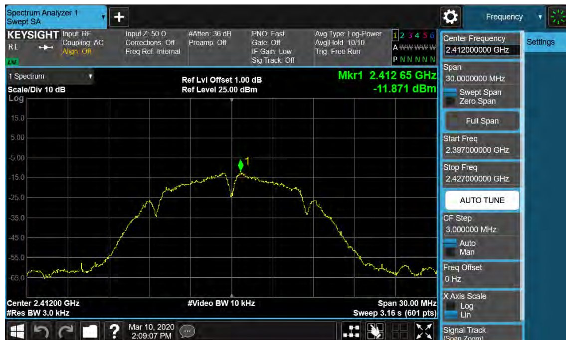
Figure 10: Power Spectral Density, 802.11b, 2412MHz
