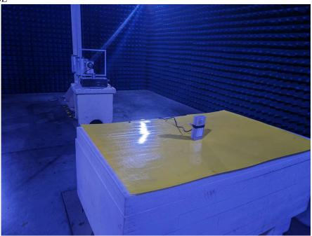
Photo of Radiated Emission Measurement (Below 1GHz)
