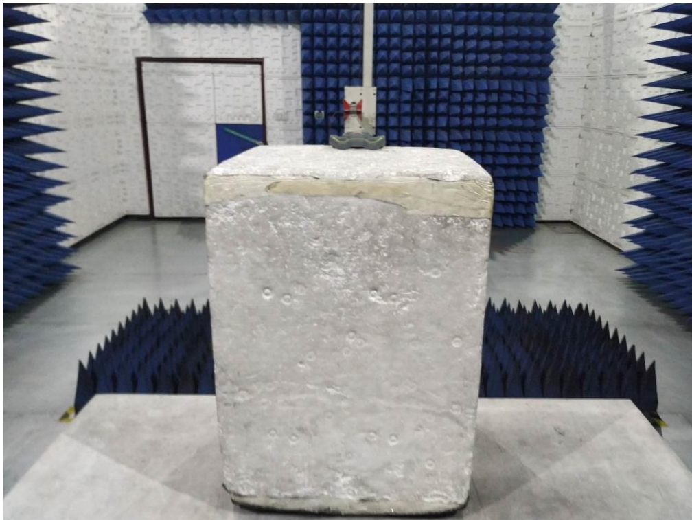
FCC RADIATED EMISSION TEST SETUP ABOVE 1GHZ
