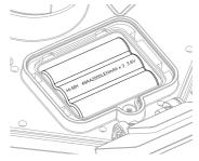
Step 5: Close the battery door and tighten the screw
