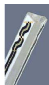
Figure 3.2 Probe Thick-Film Technique
