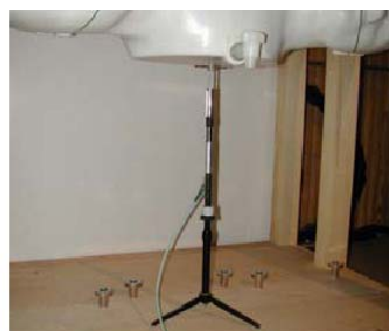
Figure 12.1 Dipole Validation Test Setup
