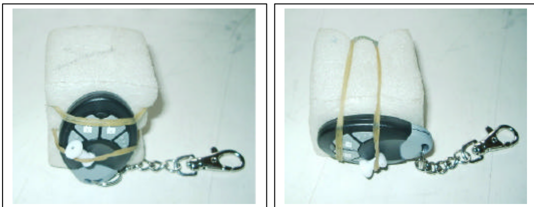
Radiated Open Site Test Set-up
