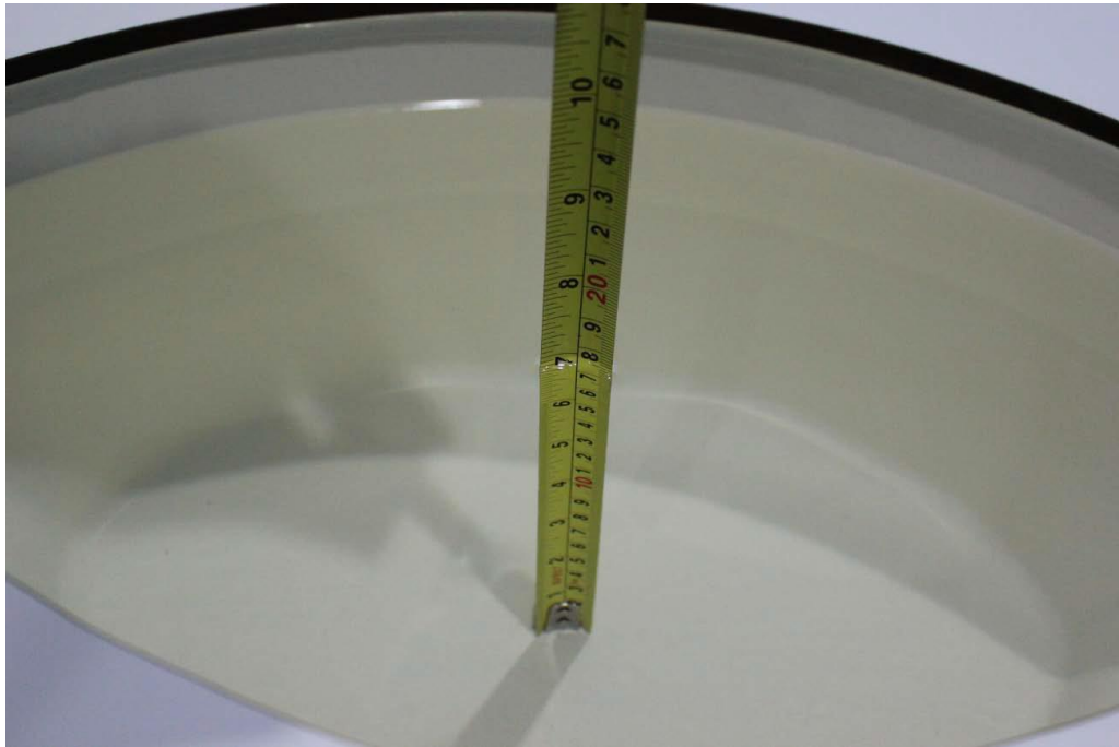
Picture 7-7: Liquid depth in the Flat Phantom(5GHz)
