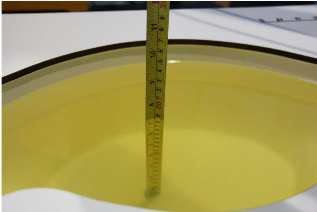
Picture 7-5: Liquid depth in the Flat Phantom(2450MHz)
