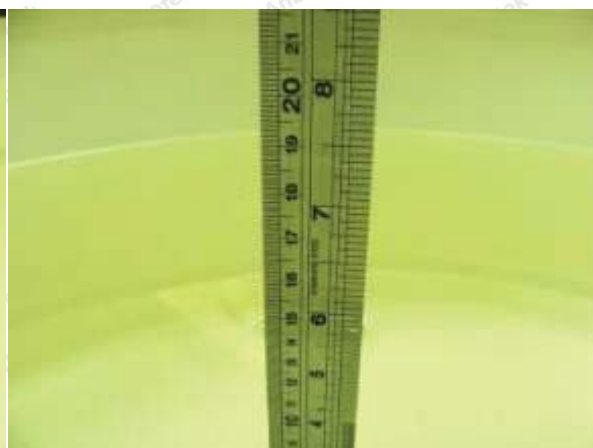
Photo of Liquid Height for Body SAR
