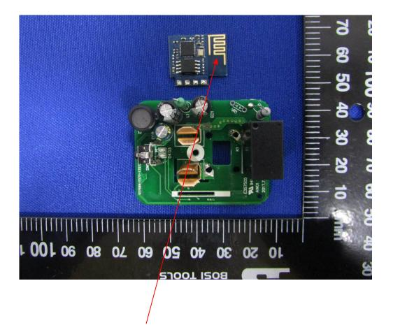
This is a PCB antenna, antenna gain is 0 dBi.
