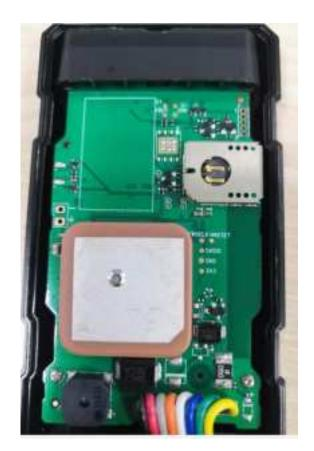
3.2 Unscrew the screw and install SIM card.
