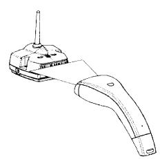
This scanner unit can now communicate with this base unit only. However, any number of scanners can be hooked up to the same MicroBar 9735 base unit. The parameters used for communicating with the base are saved to non-volatile memory in the scanner. You do not have to scan the "hook-up" badge again after changing the battery pack.
