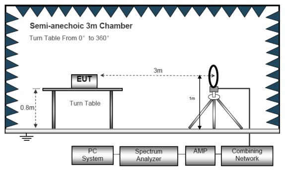
(B) Radiated Emission Test-Up Frequency 30MHz~1GHz
