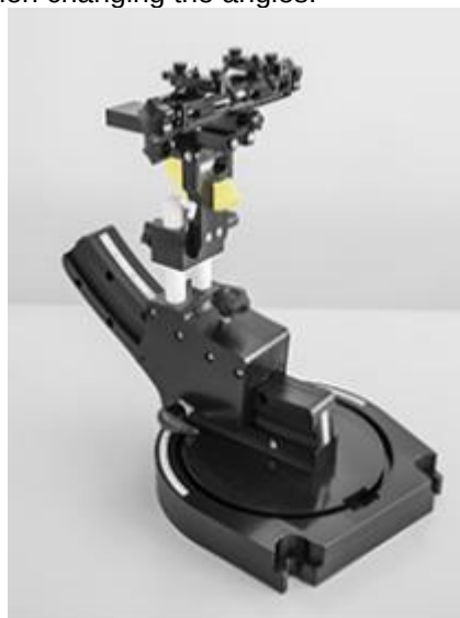
Device holder supplied by SPEAG
