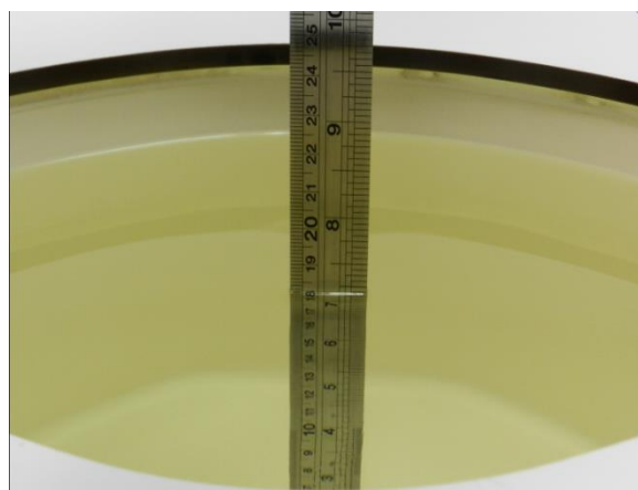
Fig 10.2 Photo of Liquid Height for Body SAR
