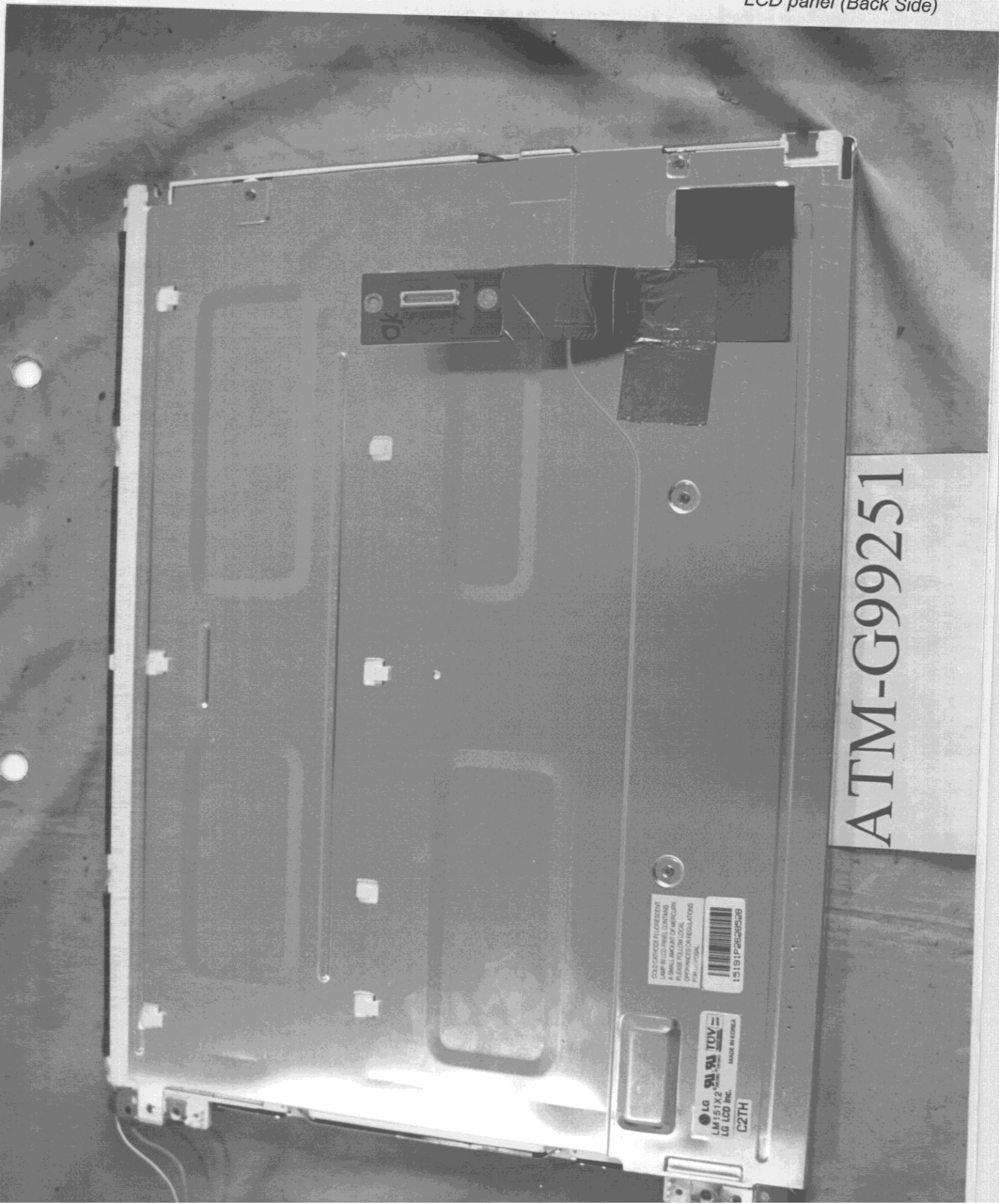
Figure 14 LCD panel (Back Side)
