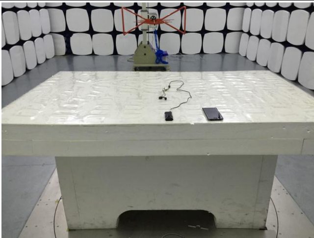
Conducted Emissions Test Setup Front View
