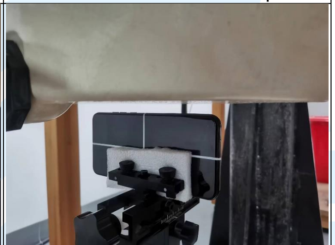
Right Side of EUT with 1.0 cm Gap
