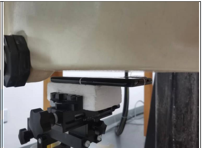
Rear Face of EUT with 1.0 cm Gap
