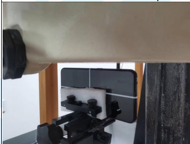
Left Side of EUT with 1.0 cm Gap
