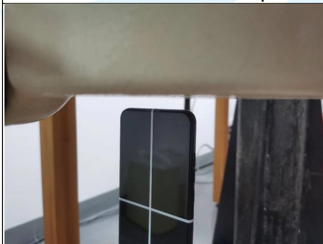
Top Side of EUT with 1.0 cm Gap
