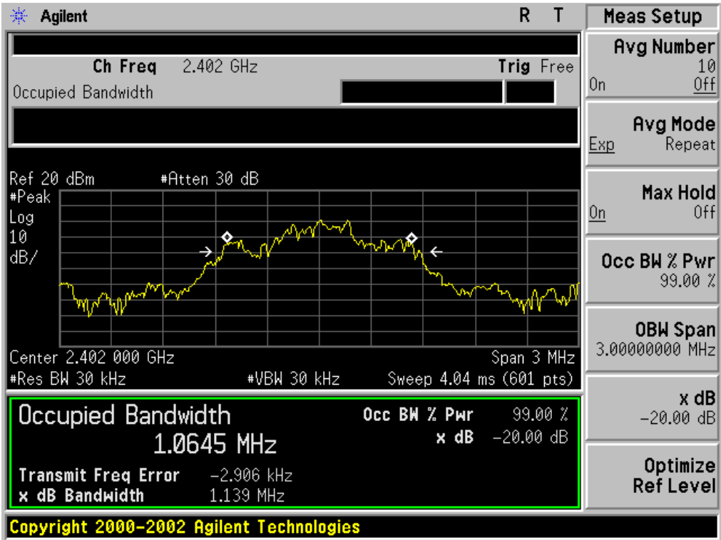
TEST PLOT OF BANDWIDTH FOR LOW CHANNEL
