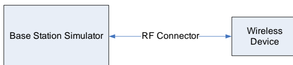
Figure 9-2 Power Measurement Setup
