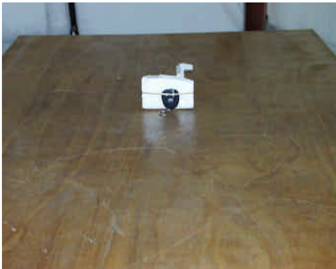
Radiated Open Site Test Set-up
