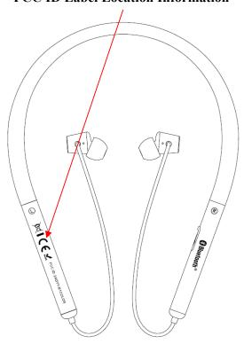
The label shown shall be permanently affixed at a conspicuous location on the device and be readily visible to the user at the time purchase (Labeling requirements per 2.925)
