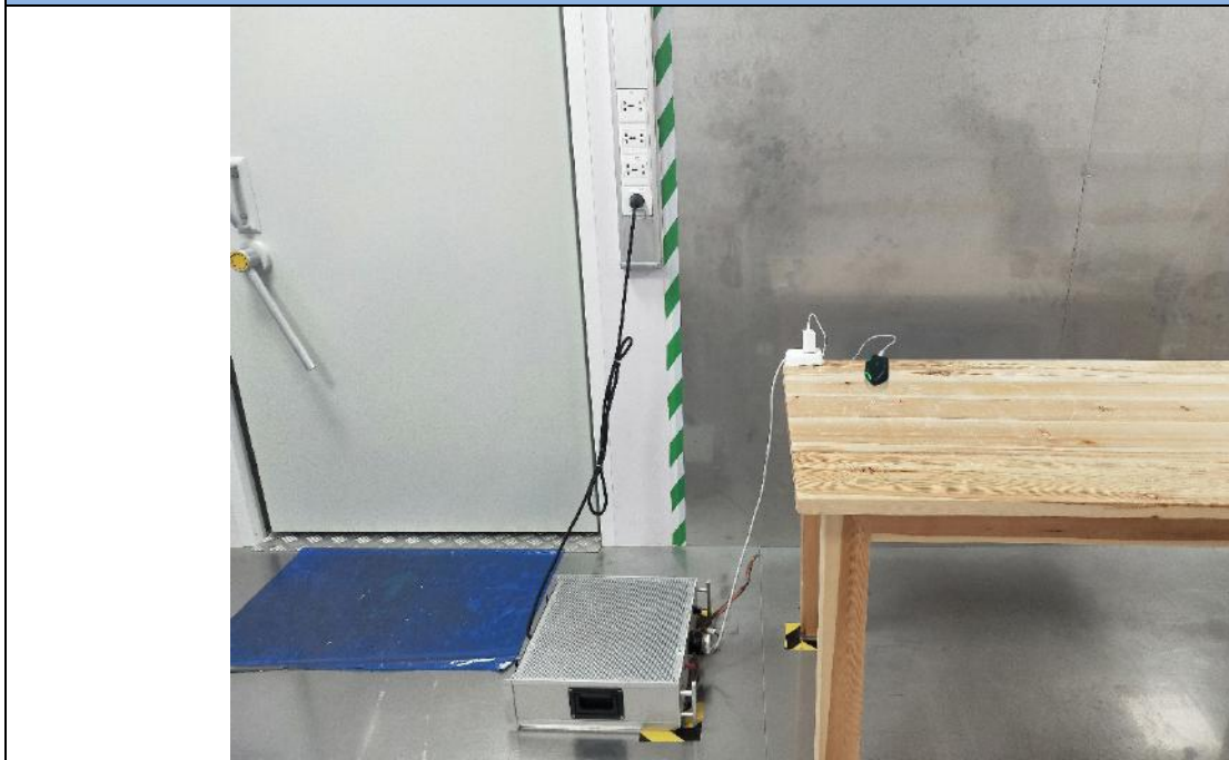
Conducted Emission at AC power line
