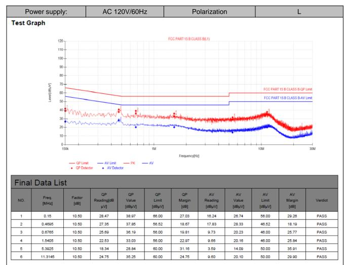
Note:1).QP Value (dBµV)= QP Reading (dBµV)+ Factor (dB)
