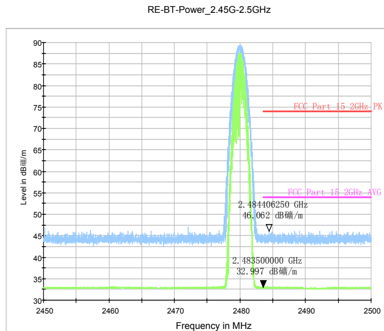
Fig.86. Radiated emission (Power): 8DPSK, high channel
