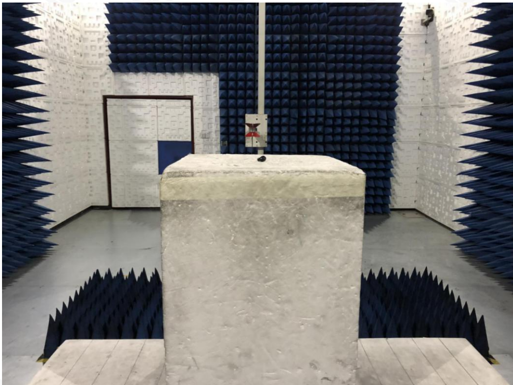
RADIATED EMISSION TEST SETUP ABOVE 1GHZ
