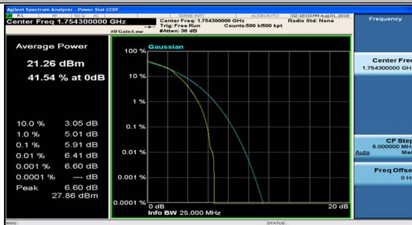
(Channel Bandwidth: 1.4 MHz)_HCH_16QAM_3RB#2
