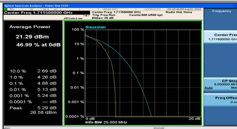
(Channel Bandwidth: 3 MHz)_LCH_QPSK_8RB#0
