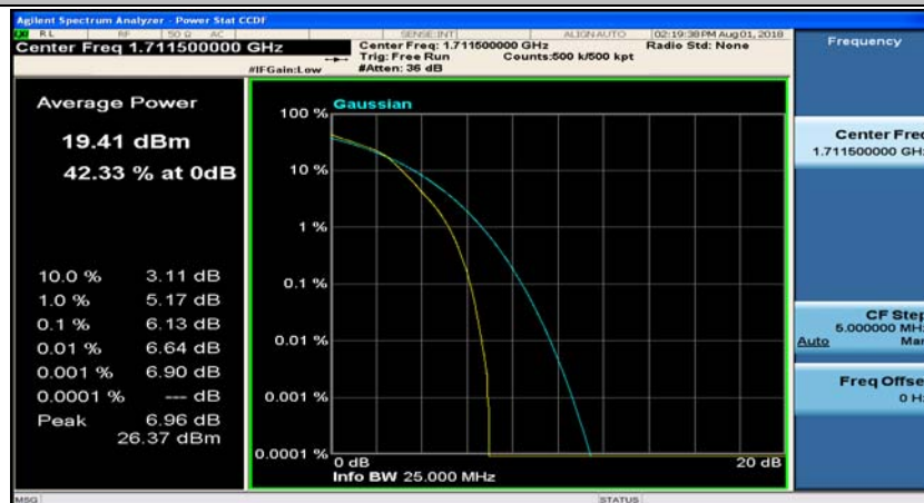
(Channel Bandwidth: 3 MHz)_LCH_16QAM_15RB#0
