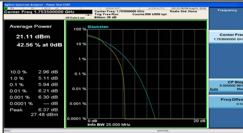
(Channel Bandwidth: 3 MHz)_HCH_16QAM_8RB#0
