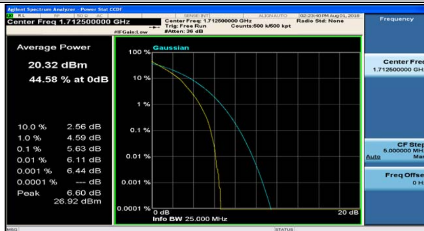
(Channel Bandwidth: 5 MHz)_LCH_QPSK_25RB#0
