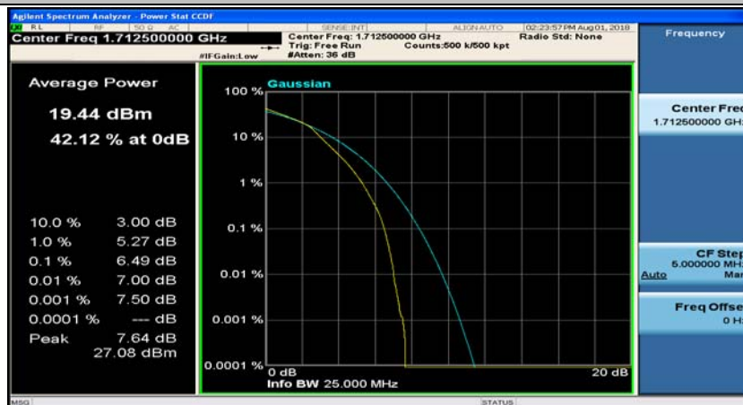
(Channel Bandwidth: 5 MHz)_LCH_16QAM_25RB#0
