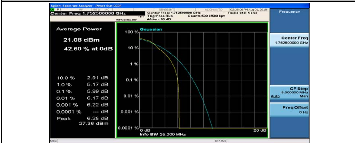
(Channel Bandwidth: 5 MHz)_HCH_16QAM_1RB#12
