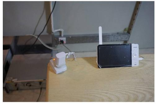
Radiated Emissions (30MHz-1GHz) Test Setup
