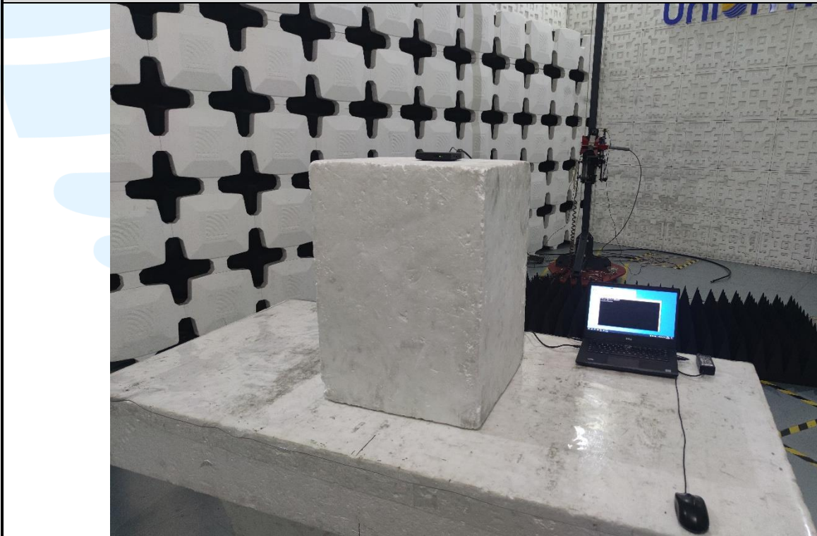
Radiated emission Test Setup (Above 1 GHz)
