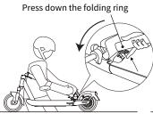
After folding down the mast, press down the folding ring, and align it with the hook on the rear end of footrest, release the folding ring to hook it successfully.
