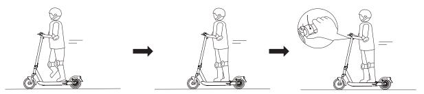
2. Stand on the footrest with one foot, the other foot kicked back on the ground and began to glide. The motor can only be started after the vehicle speed reaches 3km / h. Gently press the throttle on the right handlebar, the scooter can ride slowly, hold the handlebar to control the riding direction (similar to riding bicycle).
