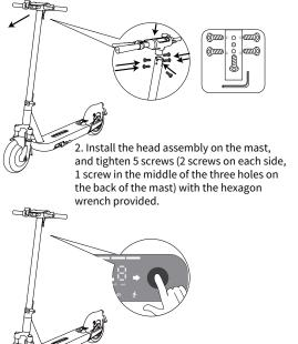
4. After installation, check the power on/off and other functions to ensure everything is normal. Check the screws again and tighten them before riding the scooter.
