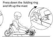
To unfold the scooter. Press down the mast, at the same time hold the folding ring until release it from the hook, and straighten the mast to ensure the folding wrench back to its position tightly.
