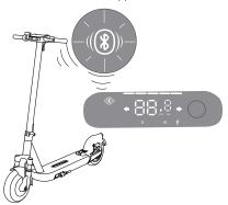
2.When the scooter turned on, by default, Bluetooth enters the status of the waiting connection. Connected the scooter with APP. The icon is always on once the connection is successful, an the user can start using the APP to operate.
