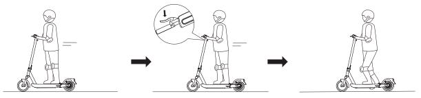
3. Gently press the throttle on the right handlebar to accelerate, but please do not be too fast. Hold the brake to make the scooter slow down (Try to avoid emergency braking). When the scooter stops or taxis slowly, get down one foot first, then get off normally.
