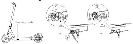
Steps: Open the cover of charging ports and plug in the charger. Cover back after charging.
