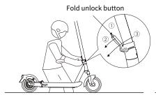
Power off the scooter, one hand hold the mast, and the other hand press the fold-unlock button and pull back the folding wrench. Then fold the mast backward.
