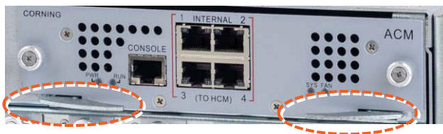
Figure 5: Module Captive Screws and Ejectors
