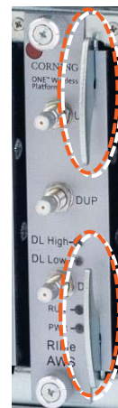
Figure 5: Module Captive Screws and Ejectors
