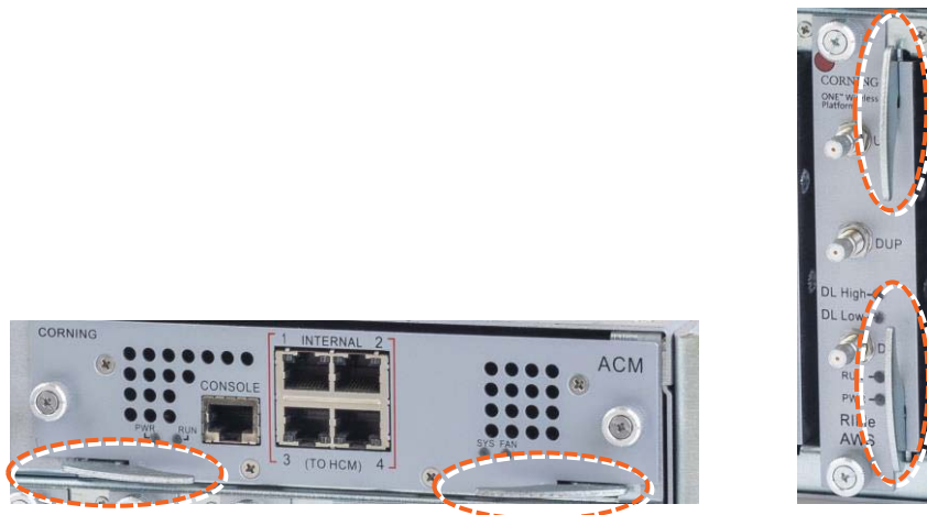
Figure 8: Module Captive Screws and Ejectors
