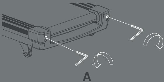
IF THE RUNNING BELT MOVES TO THE LEFT, TURN THE BOLTS ON THE LEFT SIDE ¼ OF A TURN CLOCKWISE, THEN TURN THE RIGHT BOLT ¼ TURN COUNTER-CLOCKWISE. IF THE BELT DOES NOT MOVE, REPEAT UNTIL IT CENTRES.
