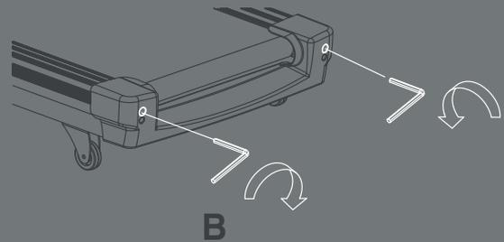
OVER TIME THE RUNNING BELT WILL LOOSEN. TO TIGHTEN THE BELT TURN THE LEFT & RIGHT SIDE BOLTS ONE FULL TURN CLOCKWISE, CHECK THE TENSION OF THE BELT. CONTINUE PROCESS UNTIL BELT IS THE CORRECT TENSION. ENSURE TO ADJUST BOTH SIDES EQUALLY TO CORRECT BELT ALIGNMENT
