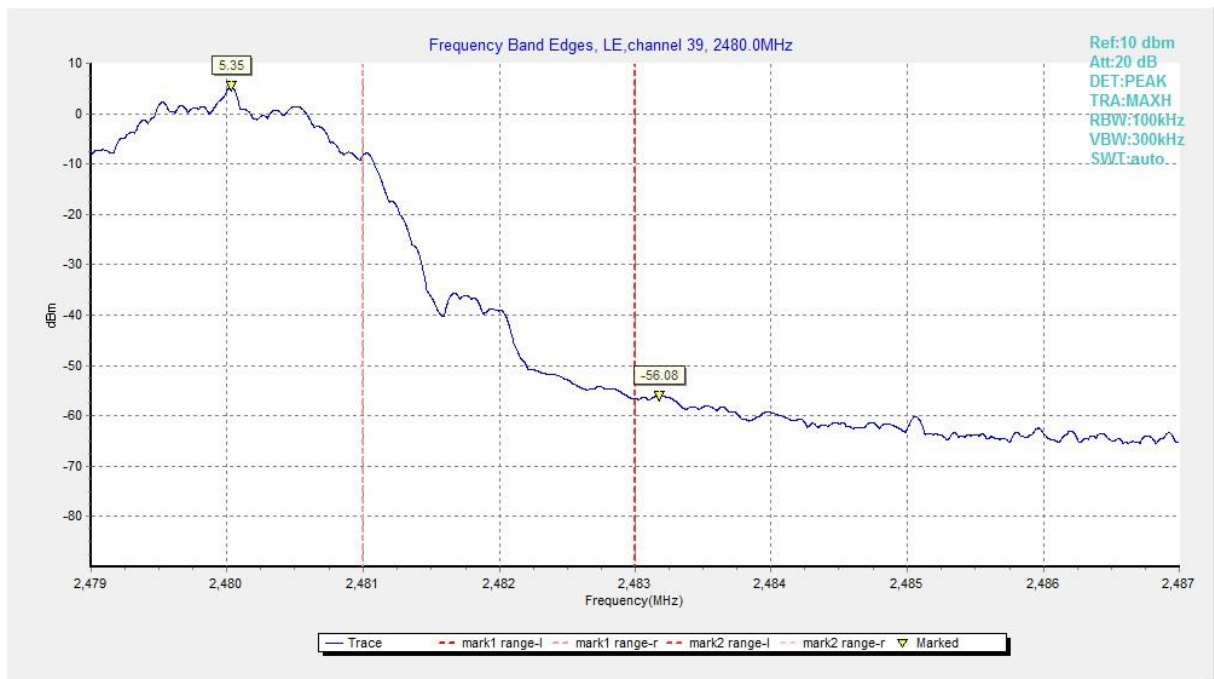
Fig.16 Band Edges (Ch 39), LE 2M
