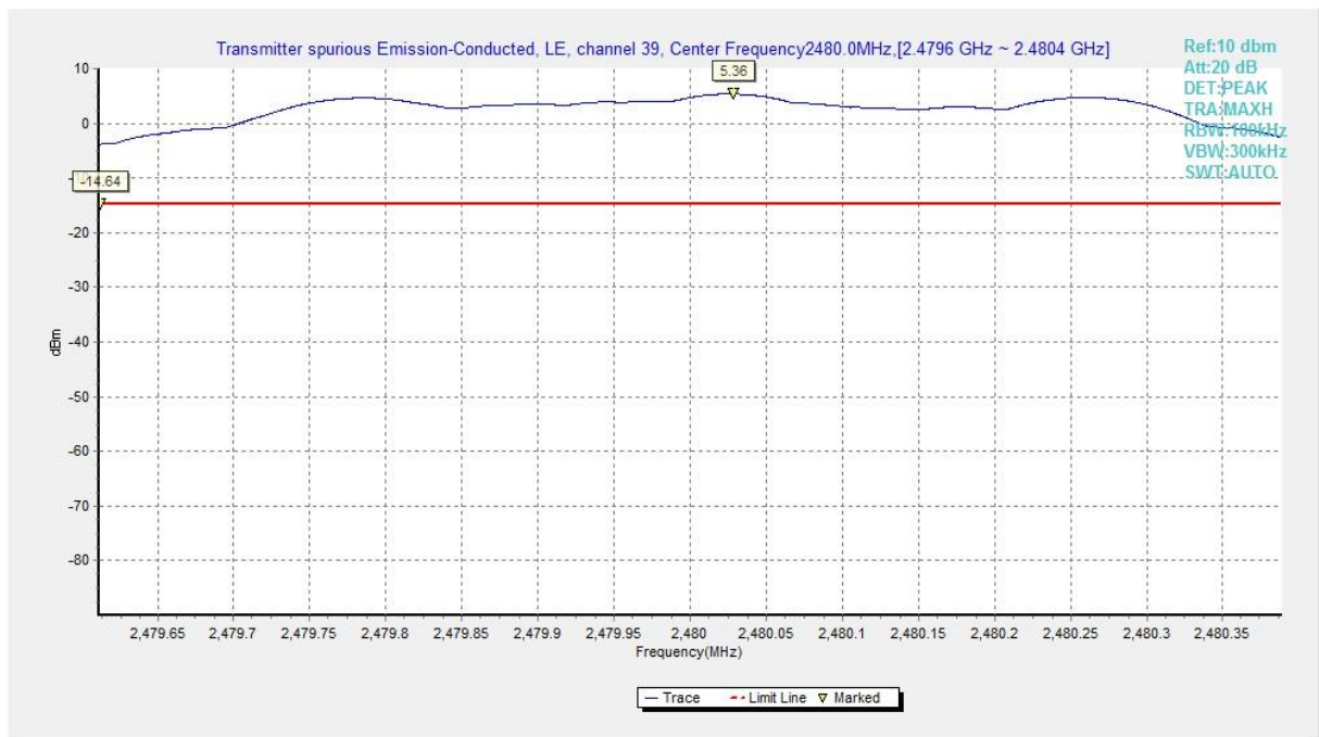
Fig.23 Conducted Spurious Emission (Ch39, Center Frequency), LE 1M
