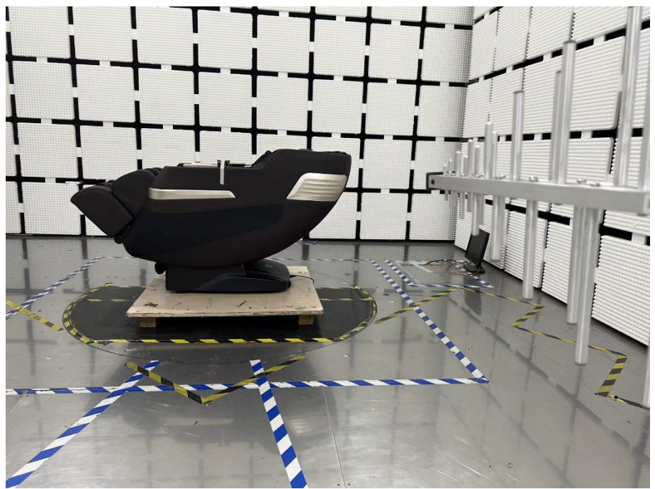
Radiation Emission Test Setup (30MHz to 1GHz)
