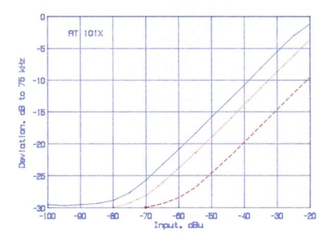
SOLID LINE: 15 kHz LONG DASH: 1 kHz SHORT DASH: 300 Hz
