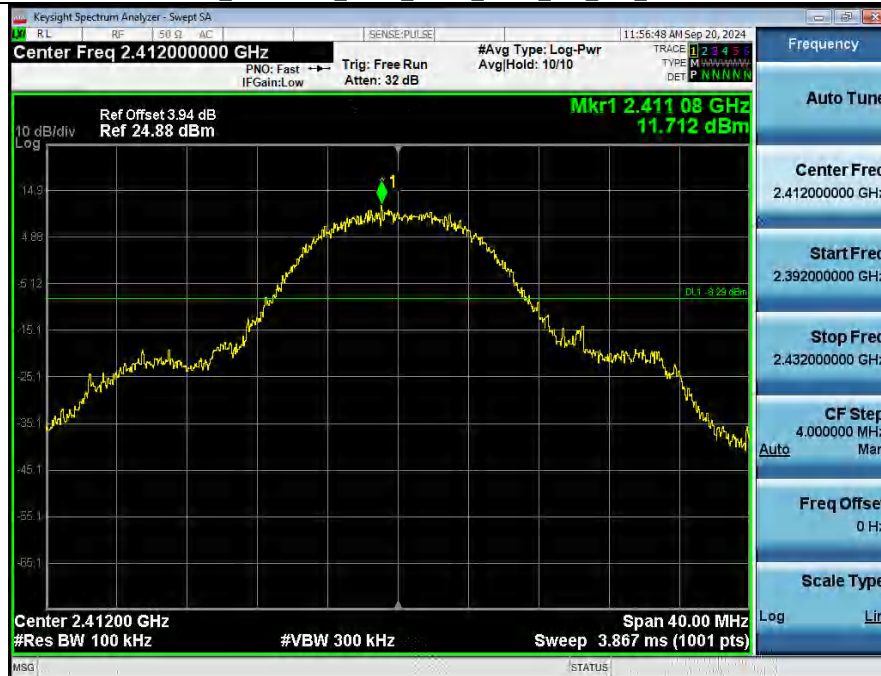
2 Spurious Emission NVNT ANT1 802_11b 2412
