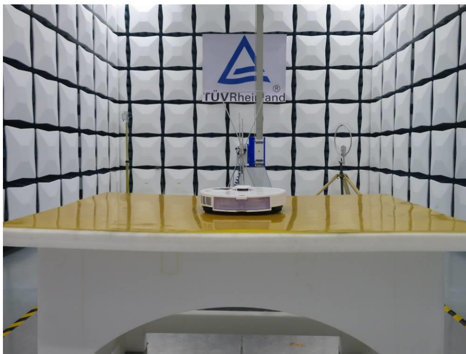
Photograph 1: Set-up photo for Radiated Spurious Emission, up to 1GHz
