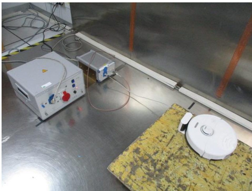
Photograph 3: Set-up photo for Conducted Emission
