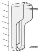
3. Drive the screws into the anchors, or directly into your wall until the bracket is tightly fastened on your wall.
