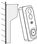
5. Attach your doorbell to the mounting bracket. Make sure it reaches the bottom where you can hear a click.
