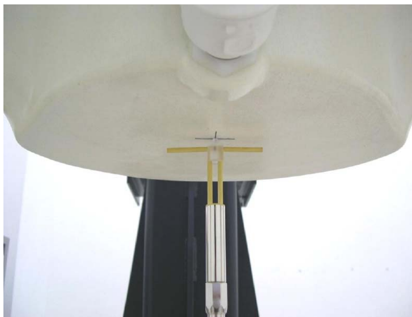
Picture 8.2 Photo of Dipole Setup
