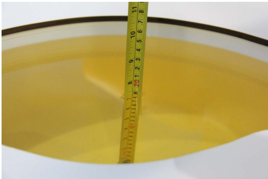
Picture 7-1 Liquid depth in the Flat Phantom (835 MHz)
