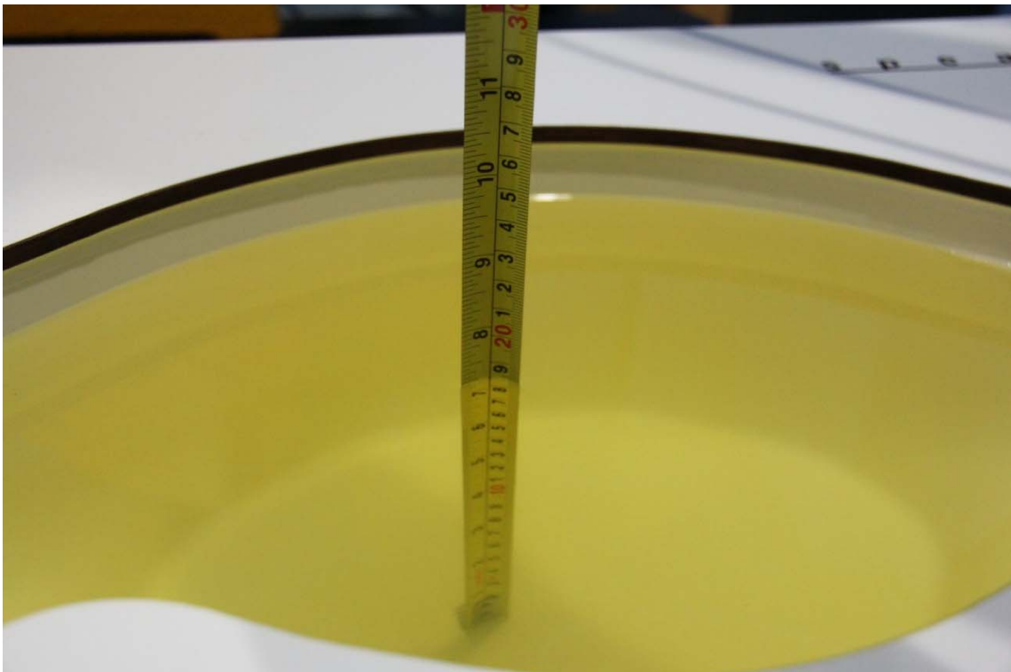
Picture 7-2 Liquid depth in the Flat Phantom (1900MHz)
