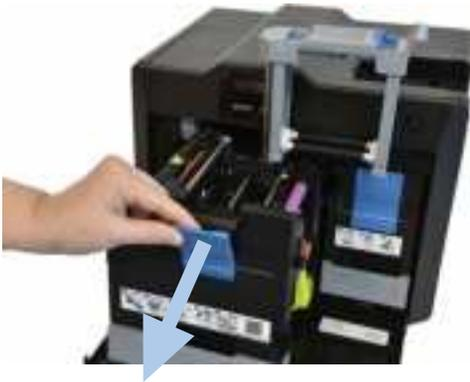
5. Load the HDP film, ensuring that each spool is correctly fitted to the corresponding color cartridge, and the film is not loose.
