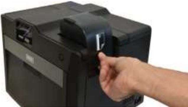
2. Load blank cards then close the card input cartridge.
