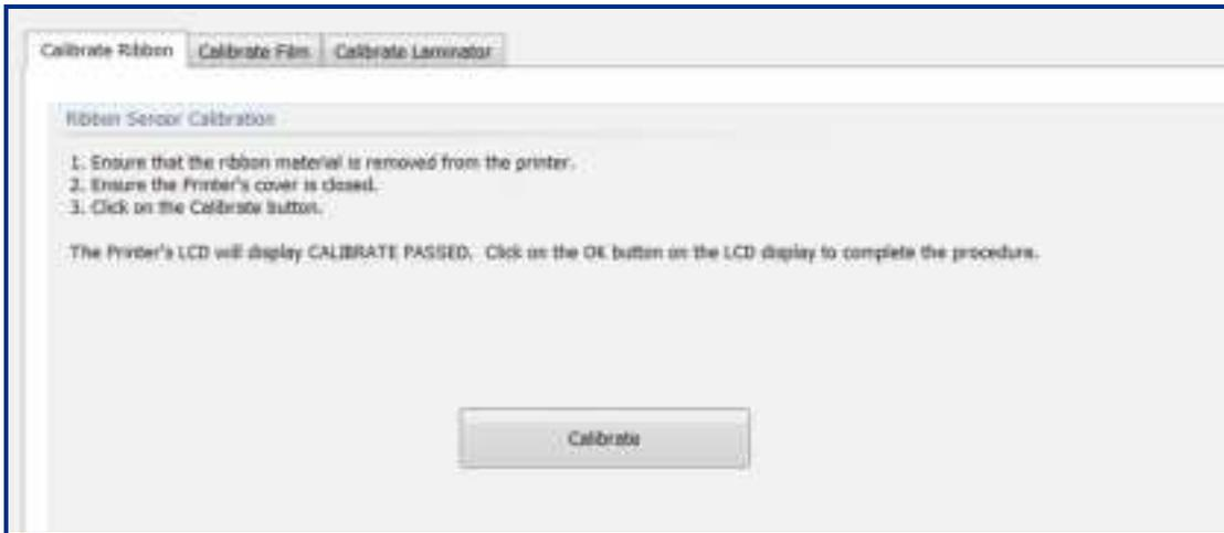
The **Calibrate Film** option sends the calibrate film command to the printer. Follow the instructions on the page for calibration of the film sensor.
