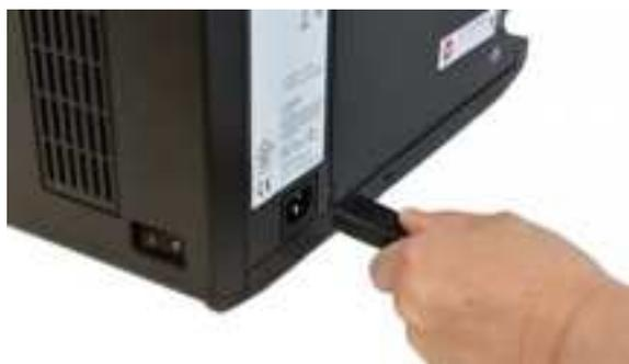
2. Plug the wall power cable into a standard 100-240 VAC power outlet.
