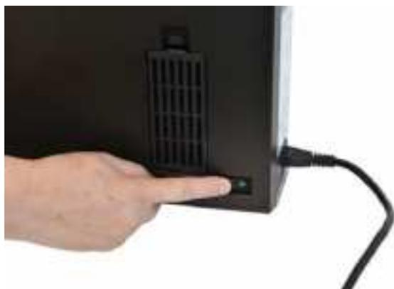
**Note:** If the physical switch is left on and the printer is left idle, the printer enters a low power state. When a print job is sent, the printer restores full power and the print job commences.
