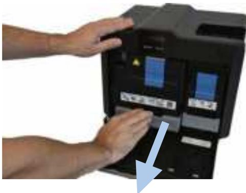
3. Unlatch and raise the accumulator unit. Twist the accumulator unit 90° to the right.
