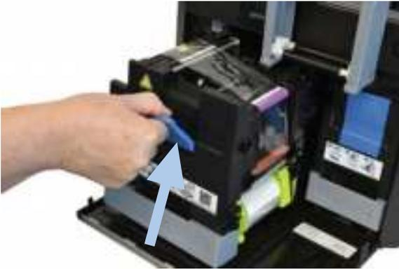
7. Twist the accumulator unit 90° to the left. Push down in the center of the accumulator unit until it clicks into place.
