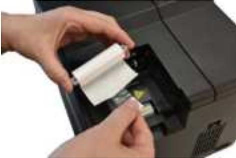
2. Insert the cleaning roller into the card input area.
